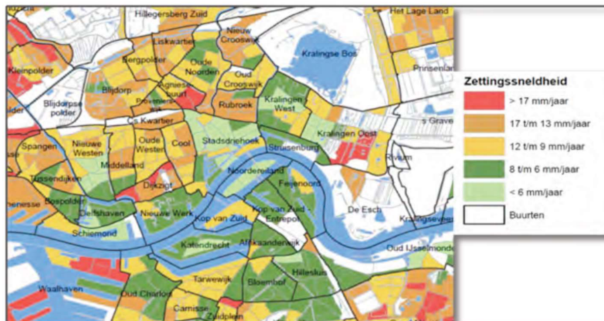
Fig 1.3.1d Soil settling / Land subsidence in mm/year.
